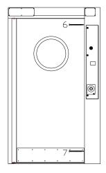
**7.** Close the door again, then fit 2 fixings into face 5 of the lock jamb.
