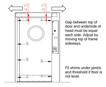
2. Working from the push side of the door, align and grip the doorset in the opening, using the frame adjusting screws A in the corners.
