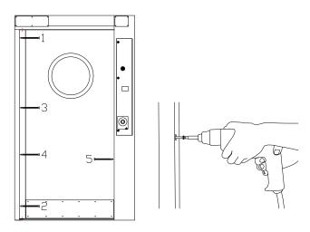
**5.** First fix as shown, with 4 fixings in the hinge jamb and 1 in the lock jamb.
