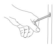
3. Tighten the frame adjusters clockwise, with a 5mm ball-ended Allen key, until the ends of the spreader plates are flat against the wall.
