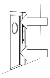
**6.** Open the door and discard the transit packings. With the door nearly closed, check the alignment between the lock edge of the door and the frame seal, at both the top and the bottom of the door.
